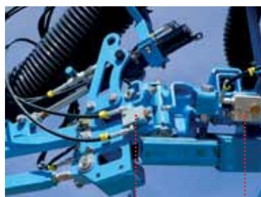
Hydraulic contactors for sequencing unfolding and spacing functions.
