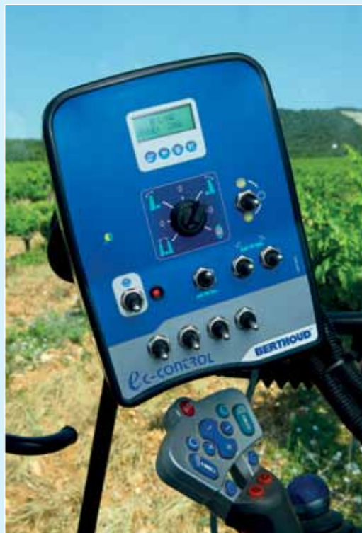
Display of volume in tank (Nivelec optional)
