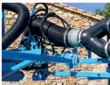
Arm support with cut-out for guiding and locking the arm in transport position.
